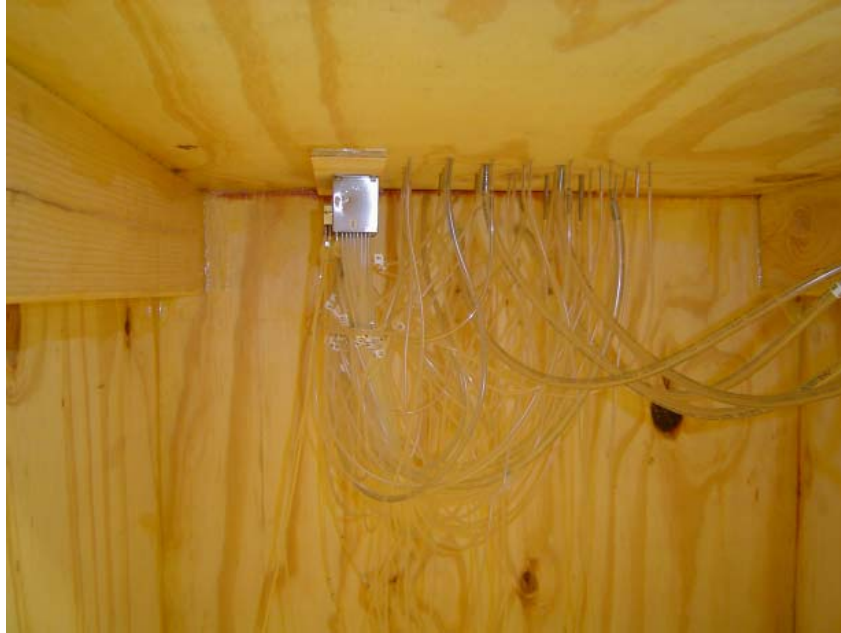
Figure 4.7. An inside view of the model showing the tube connections between the ports and the ZOC transducer
