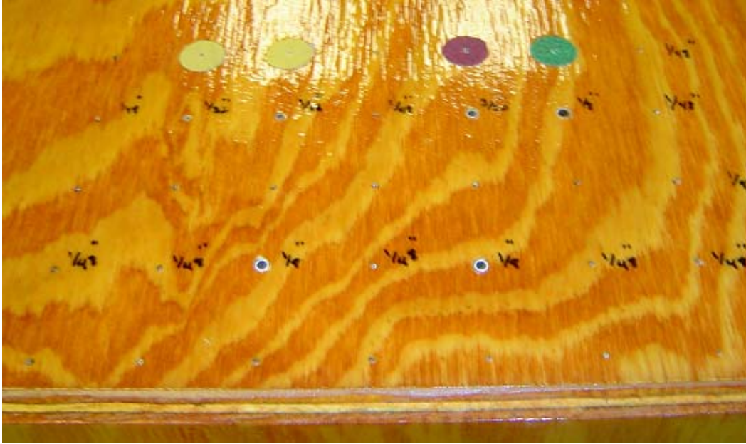
Figure 4.8. Top face of the 22 in. cube illustrating the five test rows
